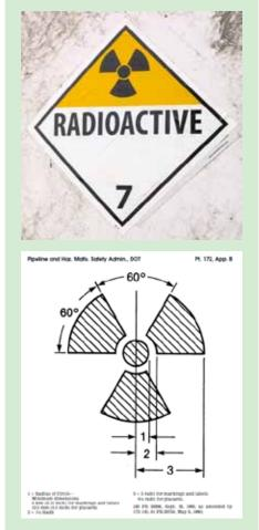
How many issues can you identify on this placard? Looking at the trefoil, does it match the allowed proportions authorized in Appendix B to 49 CFR Part 172 per 49 CFR 172.519(g)? The center dot is too big with little yellow space between the center and the blades. Also, does the package surface provide enough contrast to the placard color? If not, the placard will need either a dotted or solid line outer border to provide the needed contrast per 49 CFR 172.516(c)(7).
